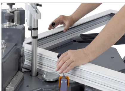
Corner crimper EP 124/20 2-hand operation
