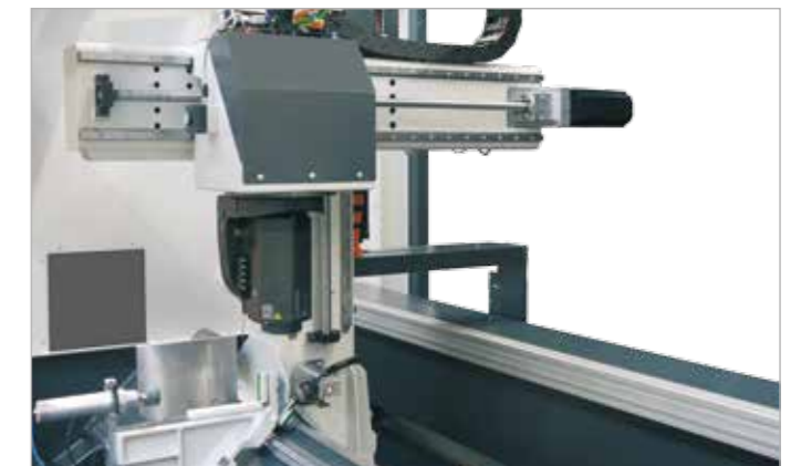
Continuously adjustable angle setting from -120° to +120° (A-axis)
