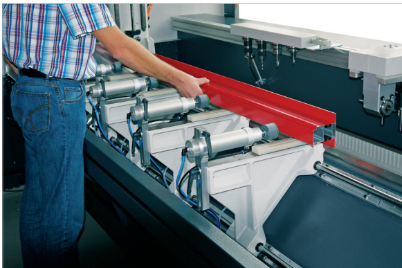
Machine bed that is executed as a modern „inclined bed“
