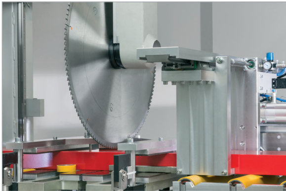
Continuously pivoting saw blade
