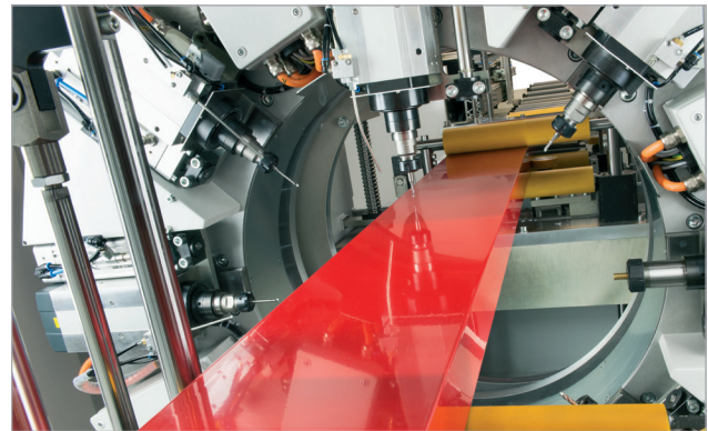
Innovative rotary module, equipped with eight spindles
