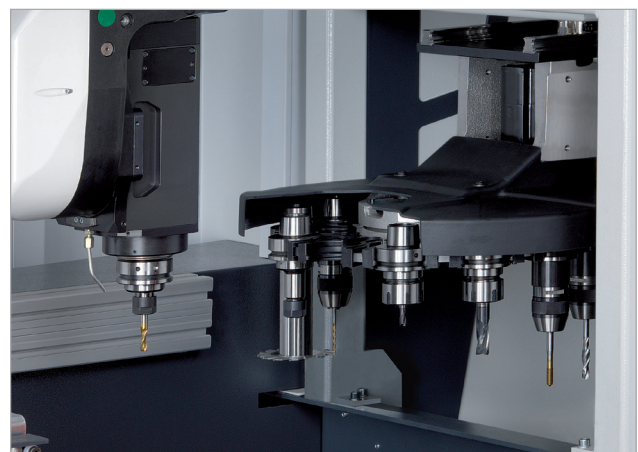
Rotating magazine with 12-fold tool changer
