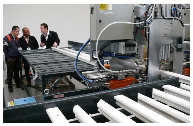
The experts were also fascinated by the SBZ 122, which is especially designed for 5-sided processing of very long profiles (up to 6.70 m in length) in metal construction, processing thick-walled profiles and tapping. They were particularly impressed with the 3-axis controller and the ability to easily program machining jobs directly on the machine using the eluCam system.
