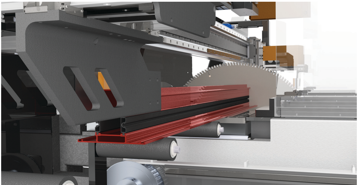
Powerful saws for aluminium and PVC profiles. The SBZ 616 variant known as the Vario, which allows for stepless and adjustable cutting angles ranging from 22.5 to 157.5 degrees.
