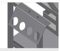
**Tool rack** Tool rack for pneumatic and electrical tools
