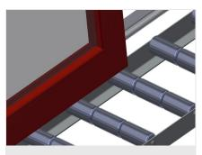
Profile protectors Profile protectors for support rollers 3x 120 mm (Alum./33 x and Alum./48 x). Support rollers covered with protective tubing
