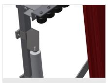
Mini-roller conveyor height adjustment
