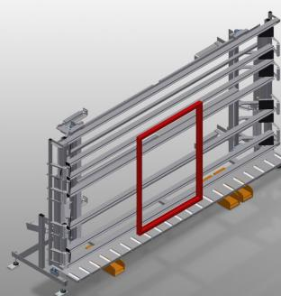
Inspection and glazing unit for glazing and final inspection in individual and serial assembly line production
