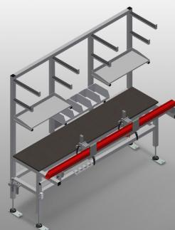
Assembly table for pre-assembly of hardware and gaskets
