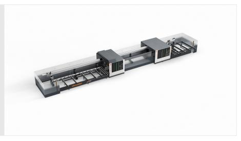
The state-of-the-art SBZ 625/13 automated pass-through centre gives users unrivalled precision and flexibility in aluminium machining. Equipped with up to 40 axes, the machining centre is durable and powerful thanks to its solid and robust design. It enables effortless machining of standard aluminium profiles and window and door profiles. Parallel machining steps significantly reduce production times, and the intuitive user interface makes it easy to use.
