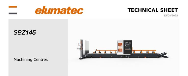
Designed for the requirements of metal construction and industrial use, the SBZ 145 with its 5 processing axes offers a processing area of 560 mm x 350 mm x 7,500mm. Equipped with an autonomous clamping axis and a generously designed tool magazine for milling cutters, drills, thread cutters and saw blades. The SBZ 145 has numerous processing options for cutting from the profile bar with processing or optionally in pendulum operation with processing of pre-cut individual parts (2x 3.250mm).
