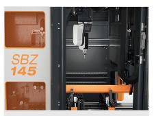
Low machine hight Low space requirement due to internal Zaxis and cable chain
