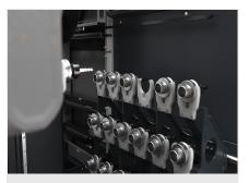
**Tool magazine** Ensures short tool change times: The horizontal, on-board mobile tool changer with 18 tool seats (3 rows of 6 tools each)
