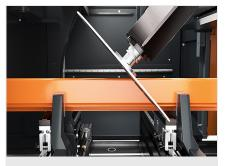
**Bar processing** Production of the individual parts from the solid bar. The individual parts are automatically pulled apart for end-face processing or notching
