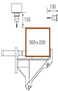
**Machining area, Y and Z-axes**
