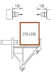
**Machining area, Y and Z-axes**
