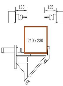
**Machining area, Y and Z-axes**
