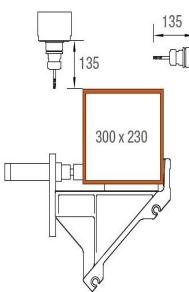
**Machining area, Y and Z-axes**
