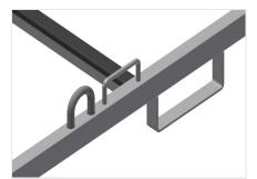
Forklift openings and crane attachment points
