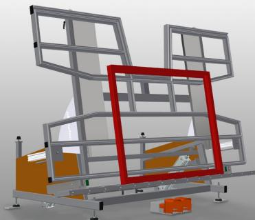
Assembly table for vertical and horizontal assembly
