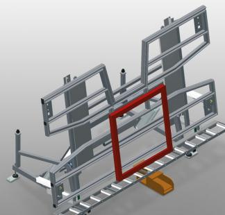
Assembly table for vertical and horizontal assembly
