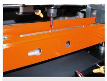
3-spindle copy router KF 178/10
