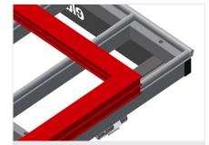
**Supporting surfaces**Supporting surfaces with plastic slide bars
