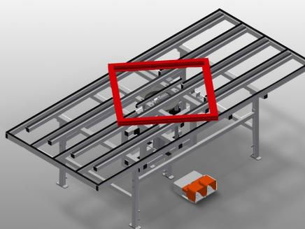
Lift and turn table for assembly and gasket insertion
