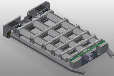
Easy handling of sheets of glass in combination with glass transport trolley GFW 15. With a pneumatic lifting unit controlled with a foot valve, max. travel = 50 mm. Lower roller conveyors equipped with 15 x 4 PVC rollers in total. Complete with draw-in mechanism for glass transport trolley GFW 15. Basic dimensions: 2.100 x 1.250 mm.
