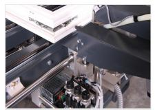
**Screwing unit**Mobile screwing unit with pneumatic height adjustment
