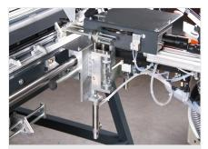
Screwing unit with mouthpiece with manual insertion funnel
