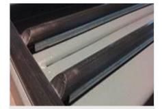
**Supporting surfaces**Supporting surfaces with plastic slide bars
