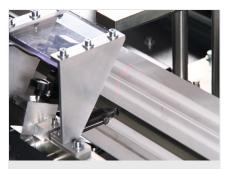
Laser unit (option) Laser for screw driving position
