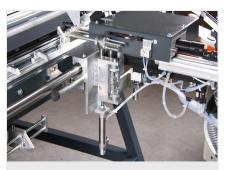
Screwing unit Mobile screwing unit with pneumatic height adjustment. Manual insertion funnel for second screw length. Automatic depth shutoff
