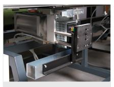
Gear cropper Gear cropper with stops for a centred and consistent handle position. Gear cropper with open cutting tool
