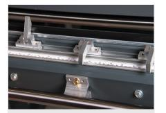
Folding stops (option) Stop rail with 14 folding stops for a consistent handle position (7x left, 7x right)
