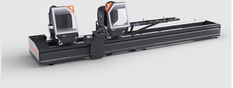
Electronic twin-head cutting-off machine with automatic traverse of the moving cutting head powered by brushless motor with numerical control system. Pneumatic control of the angular setting from 90° to 22°30' (external) in two fixed positions or with optional mechanic adjustment of intermediate angles. Hydro-pneumatic blade feed.
