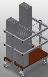
Trolley for transporting and providing a sorted selection of cut-to-length reinforcement profiles
