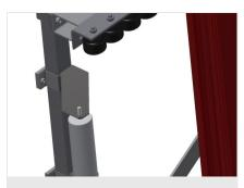
Mini-roller conveyor height adjustment
