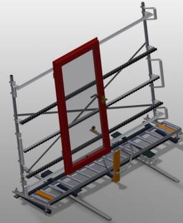
Vertical roller conveyor for transportation of window elements
