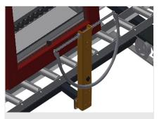
Grip makes pushing the roller conveyor on the rails easy
