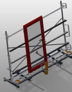
Vertical roller conveyor for transportation of window elements
