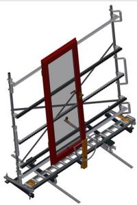
**Vertical roller conveyor VR 3000 DF with mobility and rotation mechanism**
