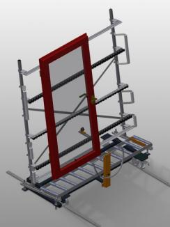
Vertical roller conveyor for transportation of window elements
