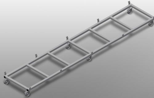
Stable steel construction. Transport trolley for carrying profile cassettes. Ideal for transporting profile cassettes from storage to the saw or to the machining centre. For profile pallets of up to 760 mm width. Safety tabs to secure the pallets. Six rollers, four swivel castors with locking stop and two fixed rollers.
