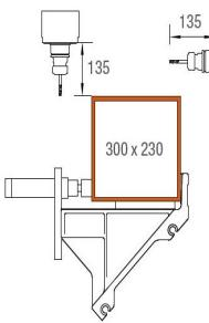
**Machining area, Y and Z-axes**
