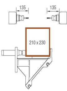
**Machining area, Y and Z-axes**
