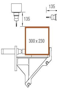
**Machining area, Y and Z-axes**
