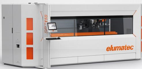
**The SBZ 118, a 3-axis profile machining centre with optional 5-sided machining that's easy to use and has a minimal footprint, expands the elumatec range of entry-level products for automated CNC machining of aluminium, PVC and thin-walled steel profiles. With its machining length of three metres, this versatile and powerful model is the most compact CNC machine in the current elumatec range.**
