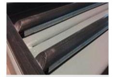
**Supporting surfaces**Supporting surfaces with plastic slide bars
