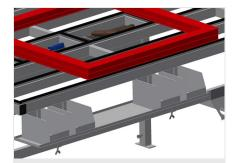
Storage area Storage area with four plastic trays for small accessories, hardware and screws
