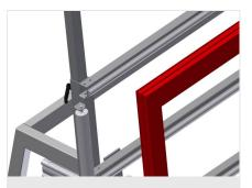
**Pull-out profile support** The table support can be pulled out at the top for MS 3000 and MS 4000 by 800 mm and 500 mm to accommodate high frames
