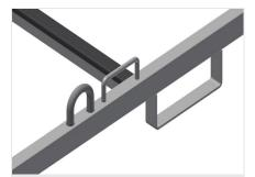
Forklift openings and crane attachment points
