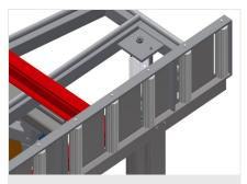
Roller support Roller conveyor can be lowered pneumatically to allow unhindered working in horizontal position; in vertical position, trouble-free onward transport is possible
