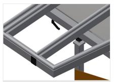
Rubber strips Supporting surfaces with rubber-knob profile
