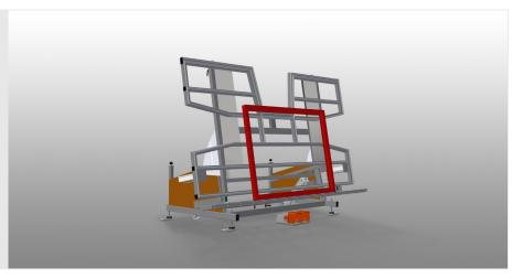
Assembly table for vertical and horizontal assembly
