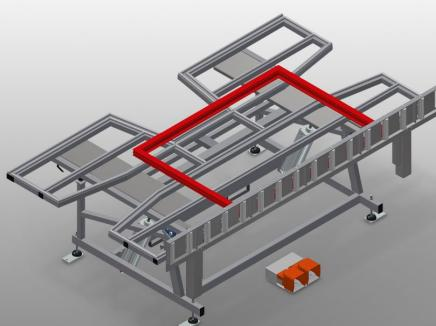
Assembly table for vertical and horizontal assembly
