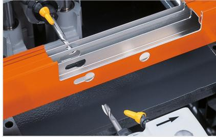
**3-spindle copy router KF
