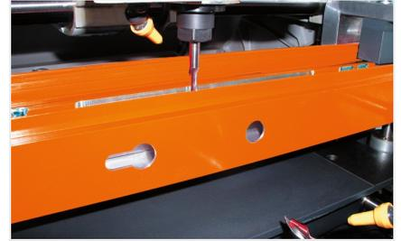
**3-spindle copy router KF
