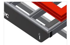
**Supporting surfaces**Supporting surfaces with plastic slide bars
