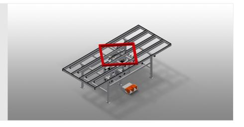
Lift and turn table for assembly and gasket insertion
