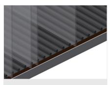
Bottom supporting surface of wood with felt
