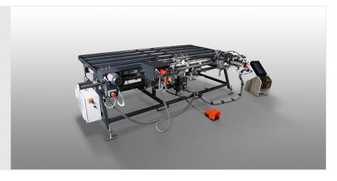
Sash assembly centre for installing hardware on PVC and aluminium window sashes
