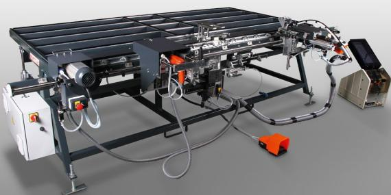
Sash assembly centre for installing hardware on PVC and aluminium window sashes
