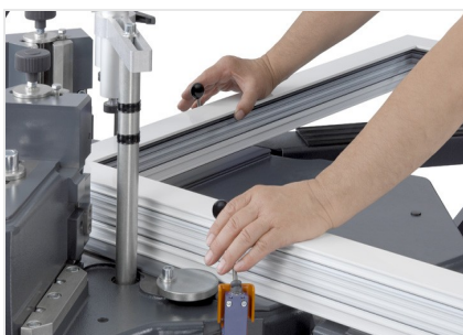
Corner crimper EP 124/20 2-hand operation
